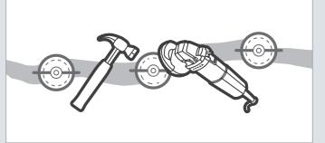
8. When epoxy is hardened, remove syringes and pedestals, and do the surface finishing work by using the hand grinder.
