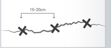
3. Mark the places which will install pedestals. The required number of syringe per one meter depends on the conditions of concrete thickness, width, depth. In most cases, 5~6 syringes per meter is appropriate.
