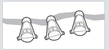
7. Suck the mixed epoxy inside syringe(30cc), and mount the syringe into pedestal, and fasten the syringe and pedestal each other using the rubber band. (Start from low area, then go to upper area. Down $\rightarrow$ Up)
